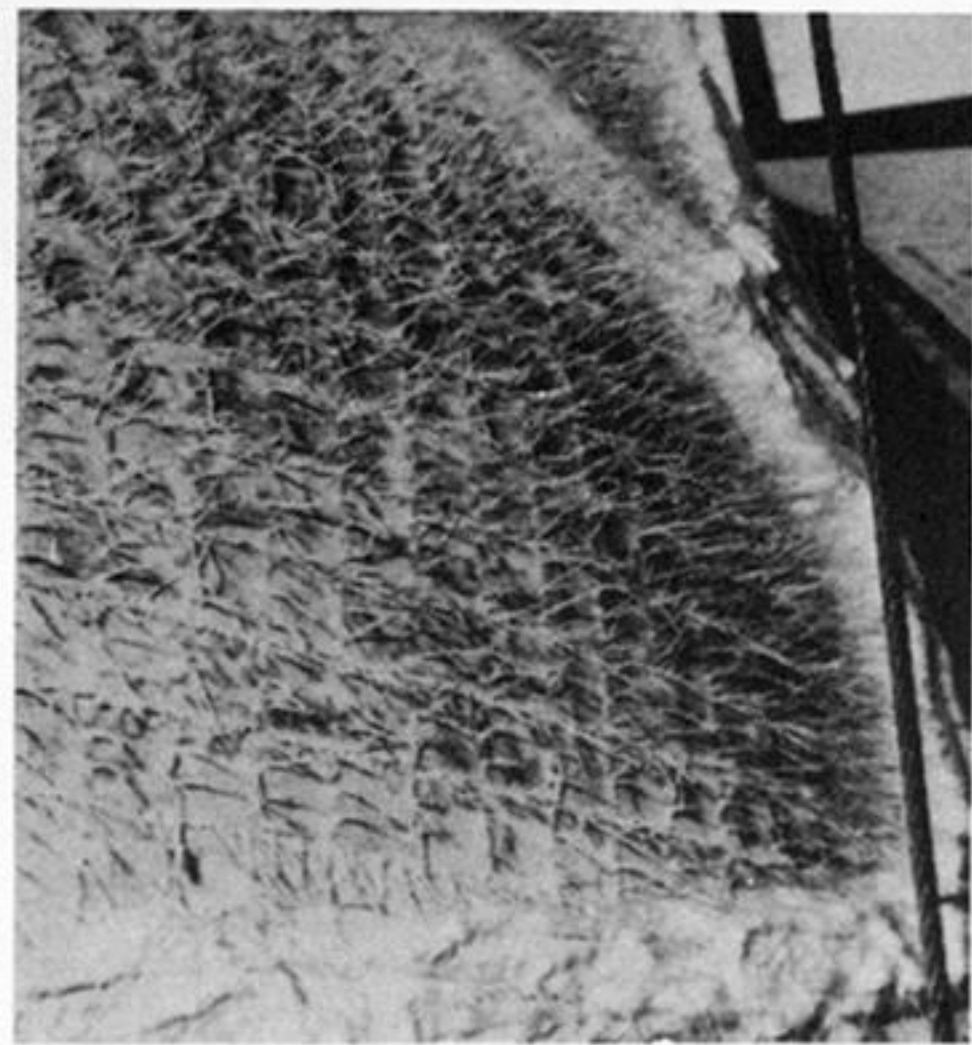
FIGURE 4. Unique aerothermal effects: blanket degradation.
